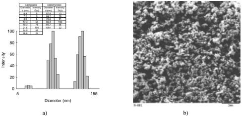
Fig. 1. a) Multimodal particle size distribution and b) SEM of unmodified TiO<sub>2</sub>
