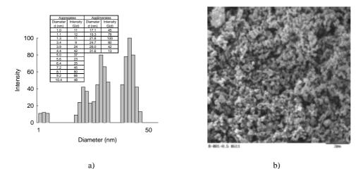
Fig. 2. a) Multimodal particle size distribution and b) SEM of TiO<sub>2</sub> modified with U-611 silane
