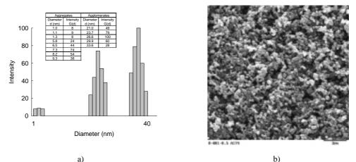
Fig. 3. a) Multimodal particle size distribution and b) SEM of  $TiO_2$  modified with A-174 silane
